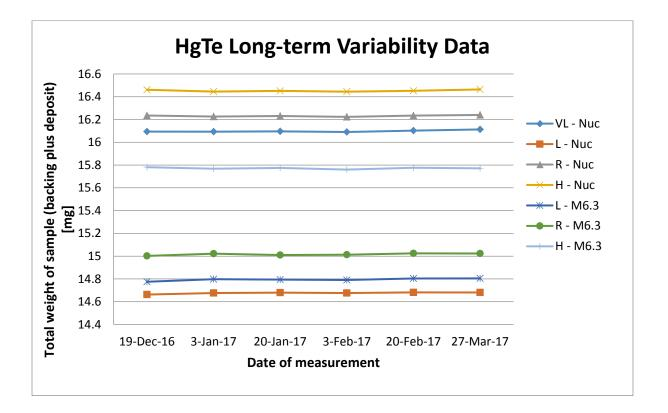
During the test period, the standards were repeatedly weighed with 0.1  $\mu$ g accuracy on a Mettler ME-30 microbalance and measured on an EDXRF analyzer at the same time points to verify the contents of Hg and Te.
