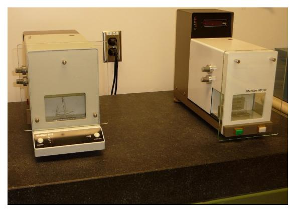
Fig. 1: Micromatter Precision Balances
