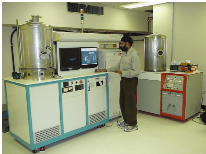
Fig. 1. TRIUMF Carbon Foil Laboratory with pulsed laser deposition system (left) and carbon arc deposition system (right).
