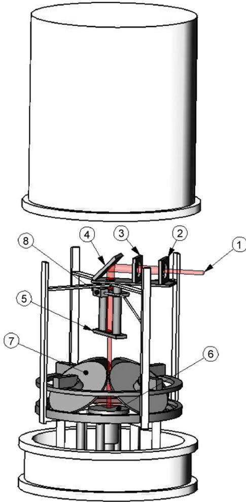
Fig. 2. Schematic drawing of the vacuum chamber of the PLD system—(1) laser beam; (2, 3) concave lenses; (4) 45° laser mirror; (5) condenser lens; (6) graphite target; (7) substrate holders; (8) crystal thickness monitor.
